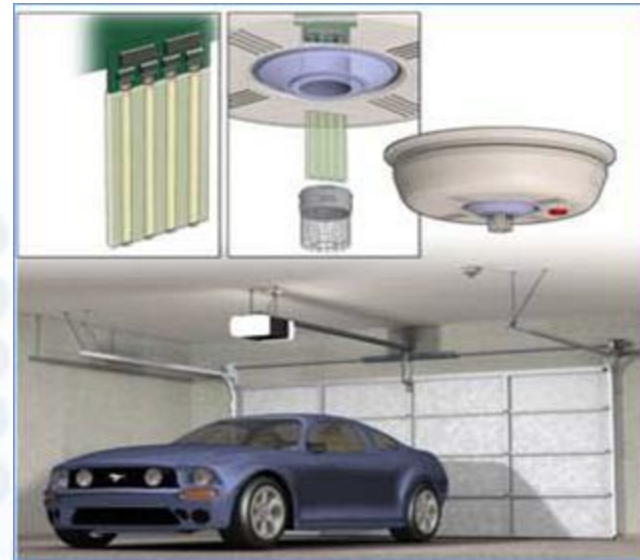
Illustration of a potential usage in civilians' car garages as a Hydrogen leak detector.
