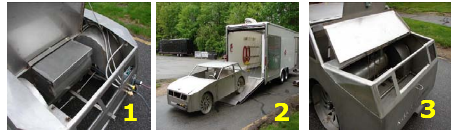
Training prop features: (1) mock fuel cell stack, (2) mobile capability, and 3) mock hydrogen storage tank.
