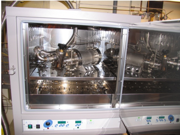
1 liter vessel under vacuum in oven
