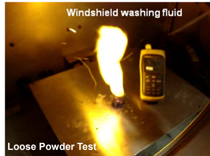
Fig.2: Windshield Washing Fluid Dropped on a Pile (0.25-gram) of Loose Powder (Vigorous Reaction with Flame Production)
