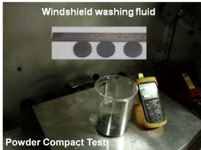
Fig.3: Powder Compact : Hydride Wafer (1-gram) Dropped in 25 ml Windshield Washing Fluid (Mild Reaction without Flame Production)
