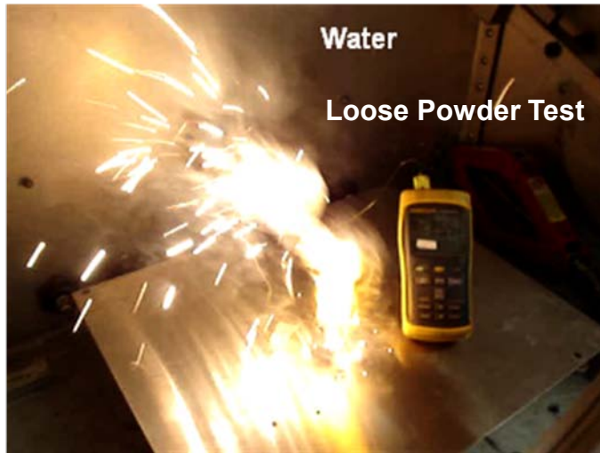
Fig.1: Water Dropped on a Pile (0.25-gram) of Loose Powder (Vigorous Reaction with Flame Production)
