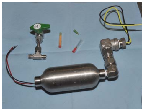
Pressure vessel used for hydrogen arcing tests
