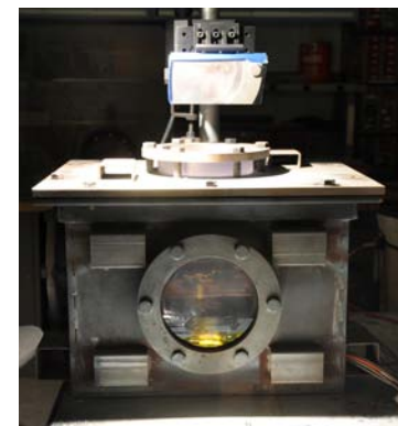
"Boom-box" borrowed from LANL nano-energetic program. Rated for 4.2 g TNT equivalent and the associated metal fragments
