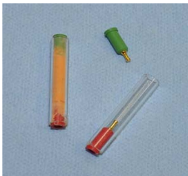
Test Cell for arcing across adsorbents in the presence of hydrogen gas (variable path 1 to 10 mm)
