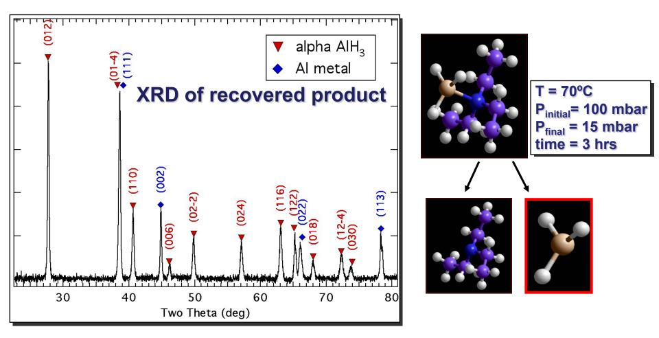
TEA-AIH<sub>3</sub> successfully separated at 70°C under vacuum (<100 mbar)</li>
