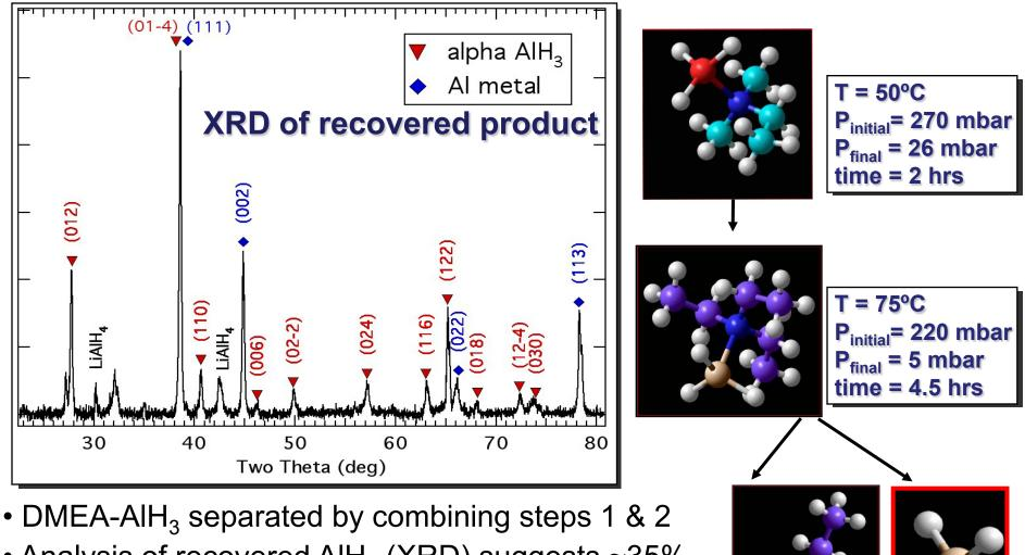
• Analysis of recovered AlH<sub>3</sub> (XRD) suggests ~35% AlH<sub>3</sub> with 65% Al when steps 1 & 2 are combined
