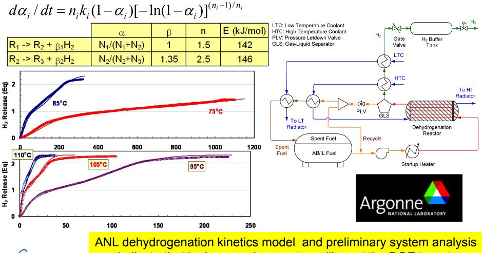
indicate that hydrogen release rates will meet the DOE target.
