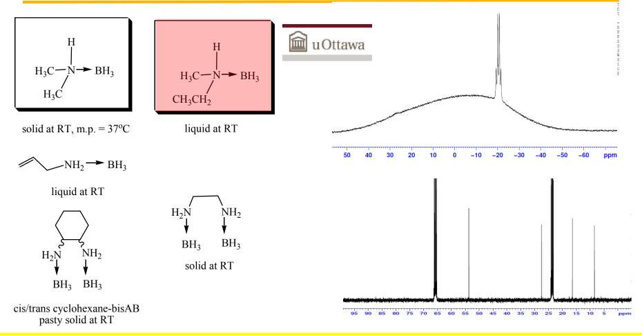
Last year sec-butylammine-BH<sub>3</sub> has shown the most promise with sec-butylammine-BH<sub>3</sub>:AB 50:50 wt% mixtures liquid at below room temp.
