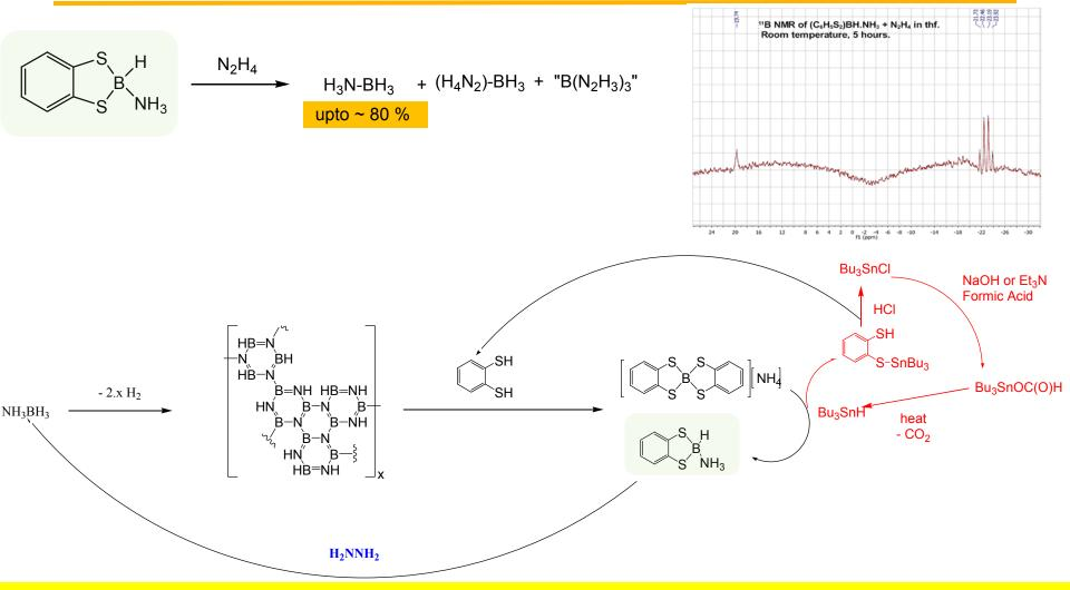
Hydrazine is a light hydrogen transfer material that removed over 50% of weight, due to tin, in the regen cycle. But some tin is still required.
