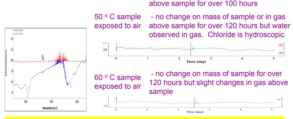
Only ammonia is observed in the gas phase at 70 C for catalyst but long term stability of samples at 60 ° C still needs to be addressed
