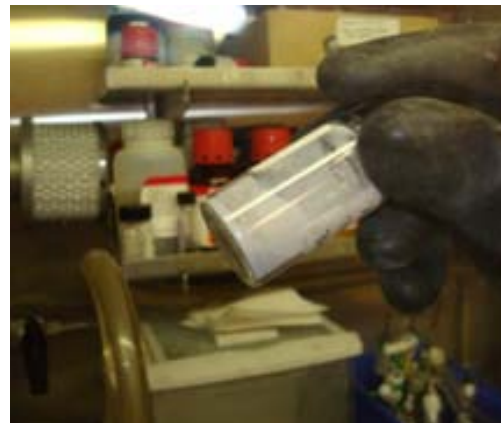
Two grams of \text{AlH}_3 electrochemically generated.
