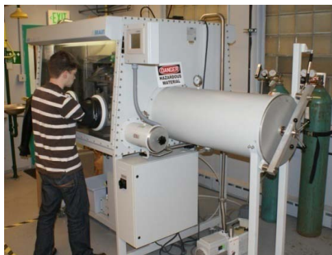
Argon filled glove-box (<0.1 ppm O 2 , <0.1 ppm H 2 O)
