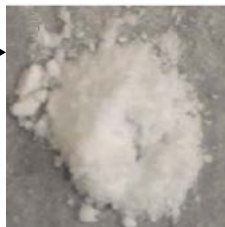
Spent product from neat AB reactor thermolysis at 120°C; summer 2009 experimental results (Basu et al.)
