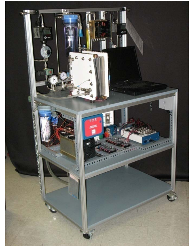
Portable fuel cell test station designed and fabricated by SERC engineers
