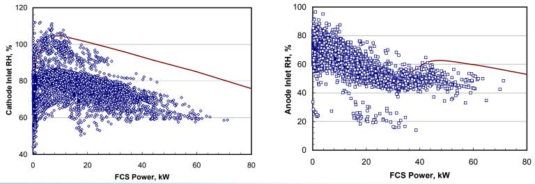
Anode humidification is due to recycle (no anode humidifier in the system)
