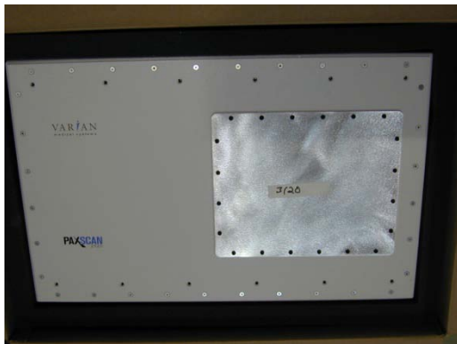
Amorphous silicon Spatial Resolution: 250 \mu\text{m} Field of View: 25 cm x 20 cm Frame Rate: 30 frame/s
