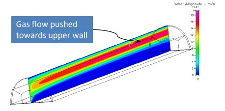
Ballard study of forward prediction of wet pressure drop, indicating extent of channel water corresponding to observed operational pressure drops
