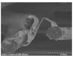
Electrophoresis treated SGL 35 AA media - 30% Teflon®
