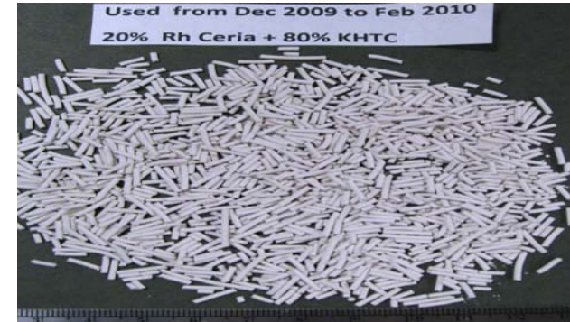
Homogenous catalyst/sorbent extrudate
