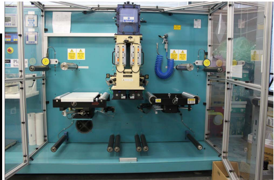
Roll to roll (R2R) coating for large area film coatings
