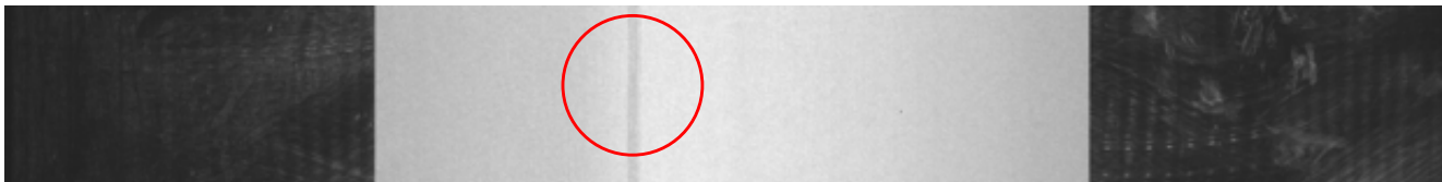
Example of a coating streak as seen in the on-line vision system
