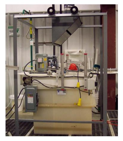
Electrodeposition Cell with newly installed exhaust system
