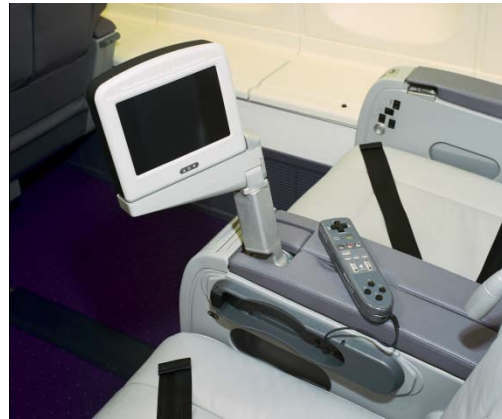
In-flight Entertainment (IFE, 20 kW) Used during all phases of flight.
