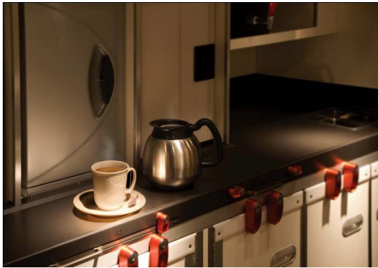
Galley (20-60 kW) Used during taxi, takeoff and climb, and cruise.
