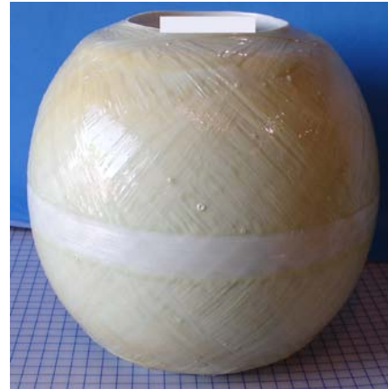
First 144" S-Glass Pressure Vessel
