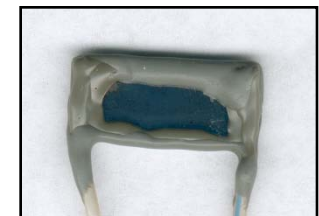
CGSe thin film after 200-hrs
