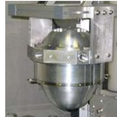
GES Electrolyzer Stack-Dome Assemblies
