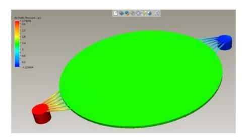
Initial computational fluid dynamics (CFD) analysis for flow passages is complete
