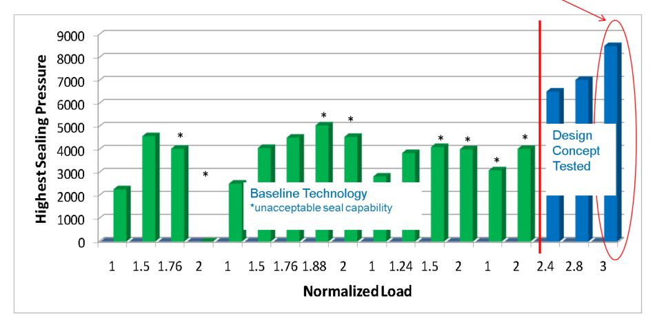
Confirmed seal integrity at elevated temperature
