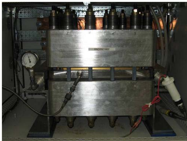
0.6 ft 2 cell stack, >10,000 cell hours, ~1 kg/day/cell
