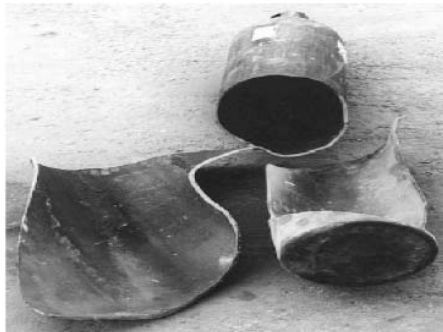
H 2 assisted fatigue of a steel tank
