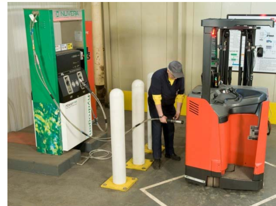
Indoor Refueling of an H 2 Fuel Cell Forklift Vehicle
