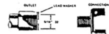
CONNECTION 110 LECTURE BOTTLE OUTLET—CORROSIVE GASES 5/16"-32 RH INT. using Flat Seal with Washer
