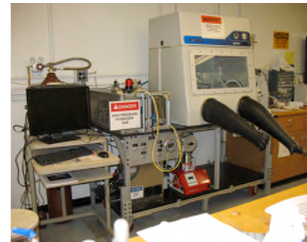
0.5-liter Hydrogen Test Fixture (HTF, Sievert apparatus, room temp.)
