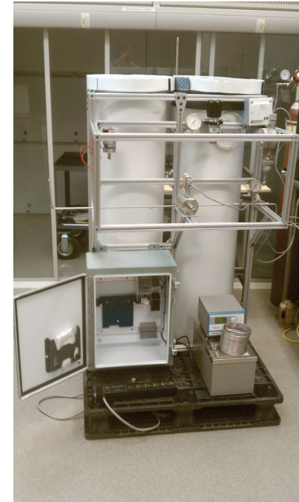
10-liter sorbent-based hydrogen tank (dry-ice temp., room temp.)
