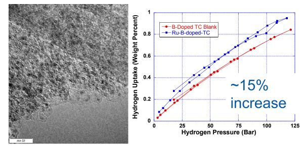
Boron substitutional materials via template (BC<sub>x</sub>), substantially improves weak chemisorption kinetics and sorption capacity
