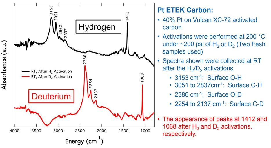
New spectral lines at 1412 and 1068 cm<sup>-1</sup> preliminarily assigned to new C-H/C-D deformation.
