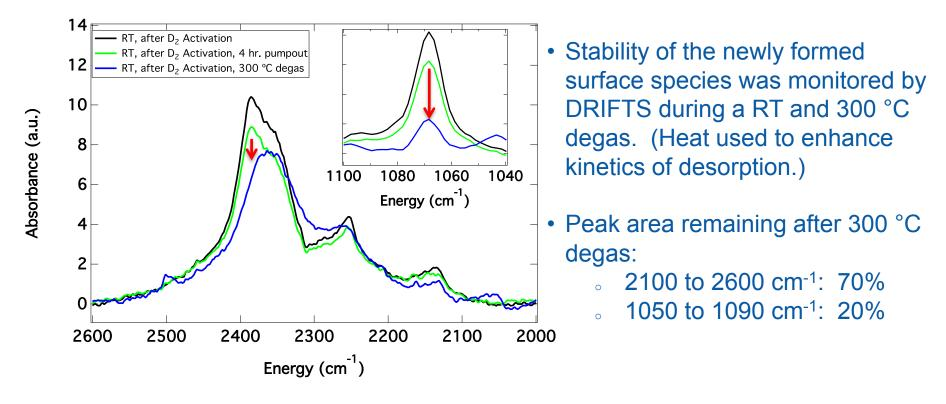
The sharp peak at 2386 cm<sup>-1</sup> disappears in concert with the 1068 cm<sup>-1</sup> peak, suggesting that the 1068 cm<sup>-1</sup> peak may possibly be due to weak C-D bonds. (Pt – D signal is >1400 cm<sup>-1</sup>)
