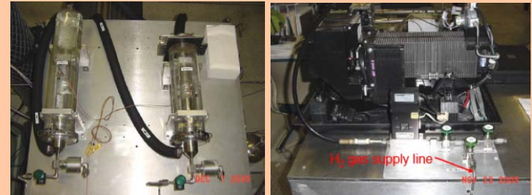
Testing an integrated MH-bed/PEM-FC hybrid power system on a facility within JPL's Hydrogen Storage Engineering Lab (HSEL)
