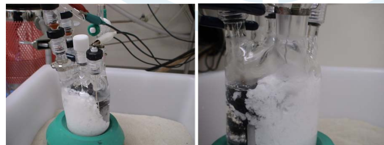
Electrochemical Cell Generating \text{AlH}_3 - TEDA
