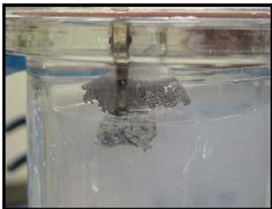
Aluminum electrode dissolved after an electrochemical run as expected when \text{AlH}_3 is formed. 5
