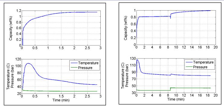
Absorption profiles for Hy-Stor 208. MmAl<sub>4.5</sub>Ni<sub>0.5</sub> at various pressures. Demonstration of rapid kinetics and acceptable H2 capacity.
