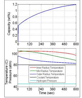
Refueling Simulation Results Showing the Full 1.2 weight % of H2 Absorbed in 10 min.
