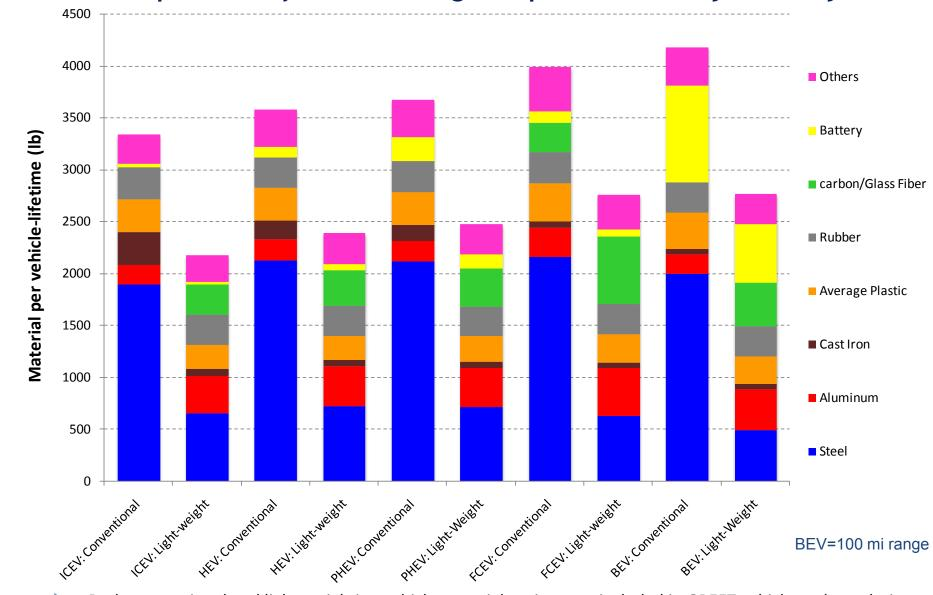
Material Composition of Vehicle Weight Impact Vehicle Cycle Analysis
