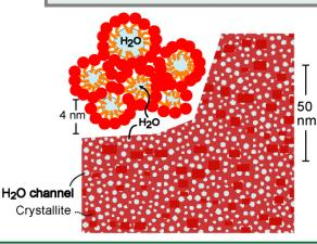
The Nanostructure of Nafion<sup>®</sup> Fuel-Cell Membrane
