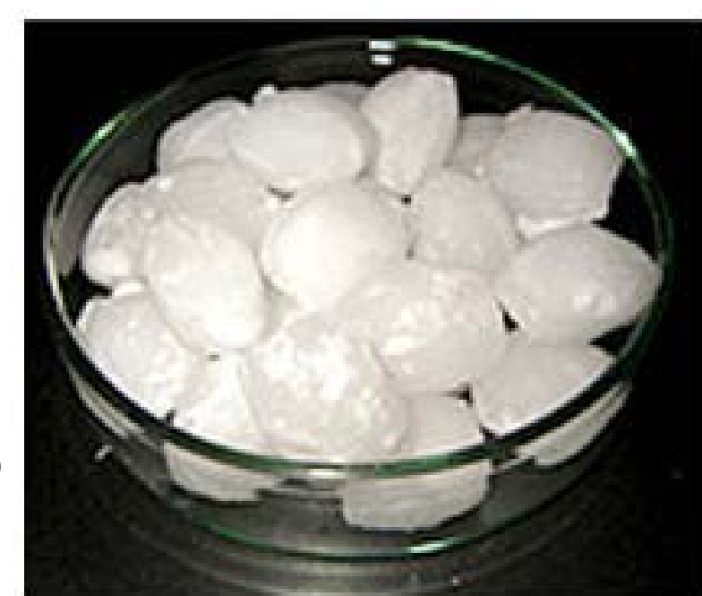
NGH Hydrate Pellets 'Self Preserved' at 1 atm, -20 °C
