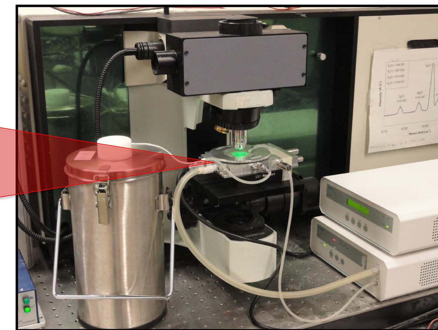
LabRAM HR confocal Raman with cooling stage
