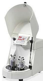
Reactive ball milling of  $\text{MgB}_2$  (in Fritsch P7 miller) at temperatures between  $-30^\circ\text{C}$ –RT and 1–350 bar pressure.
