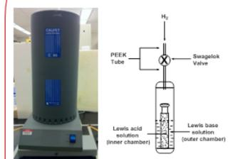
Mixing cell under ambient N<sub>2</sub> atmosphere (loading) cells in glove box) :  $\Delta H$  observed (integrated area) is combination of enthalpy of dative bond and heats of dilution
