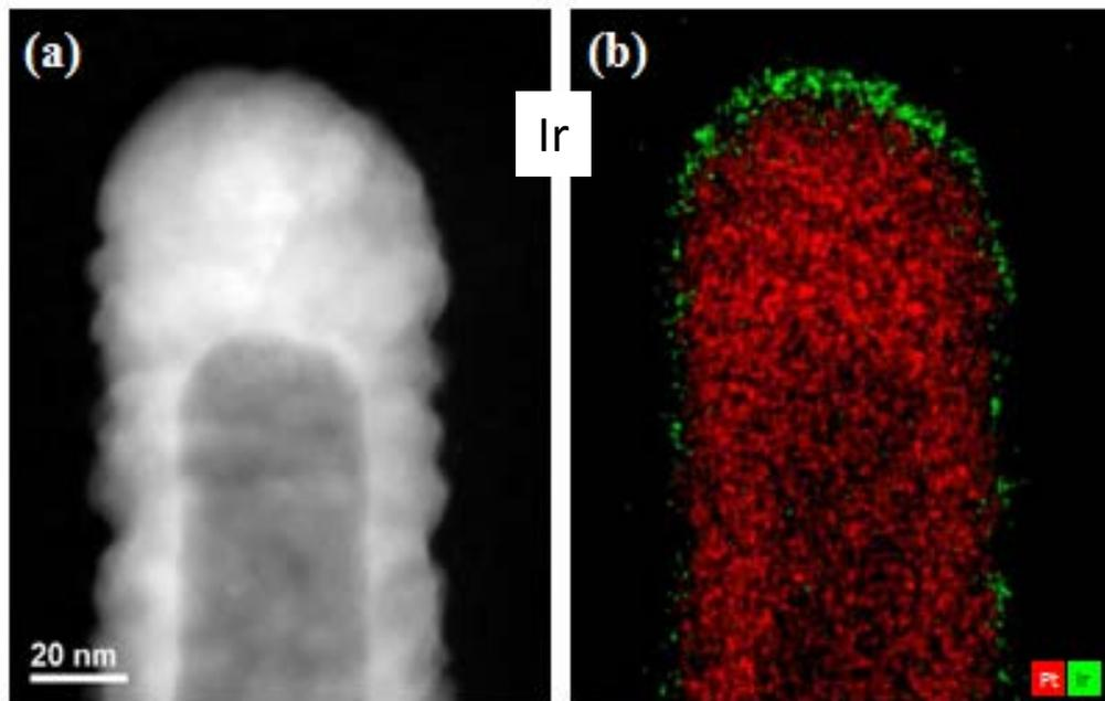
STEM (a) and EDS map (b) of Ir 10  $\mu\text{g}/\text{cm}^2$  on Pt-NSTF after FC performance tests. Nearly all the Ir remains on the whisker surface indicating Ir, unlike Ti and Ru, is stable in FC environment.
