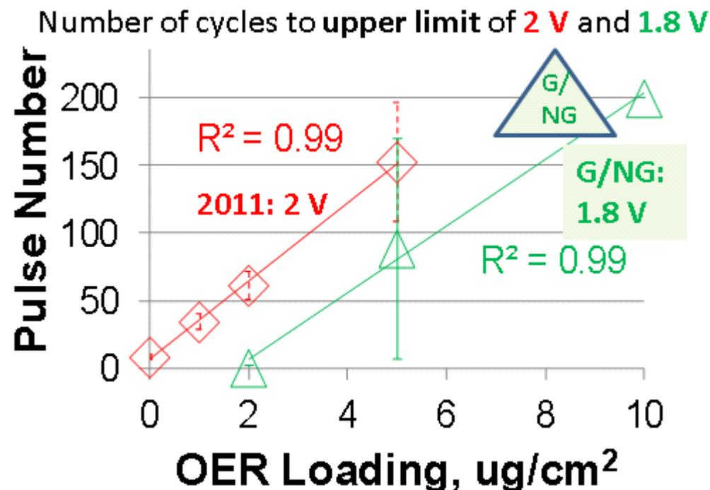
All 6 samples tested w/ 10  $\mu\text{g}$  OER have passed 200 cycles with a lot of “room” to spare. **These samples fulfilled Year 2 milestone.**
