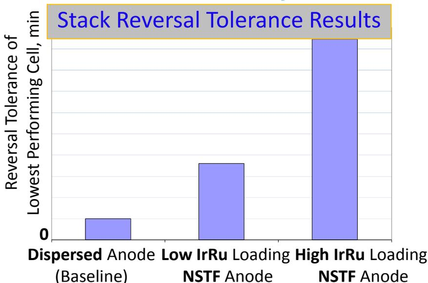
**In stacks**, as in AFCC's subscale configuration (reported in 2011 AMR) the **OER-Pt/NSTF anode consistently outperformed** dispersed baselines with higher loadings
