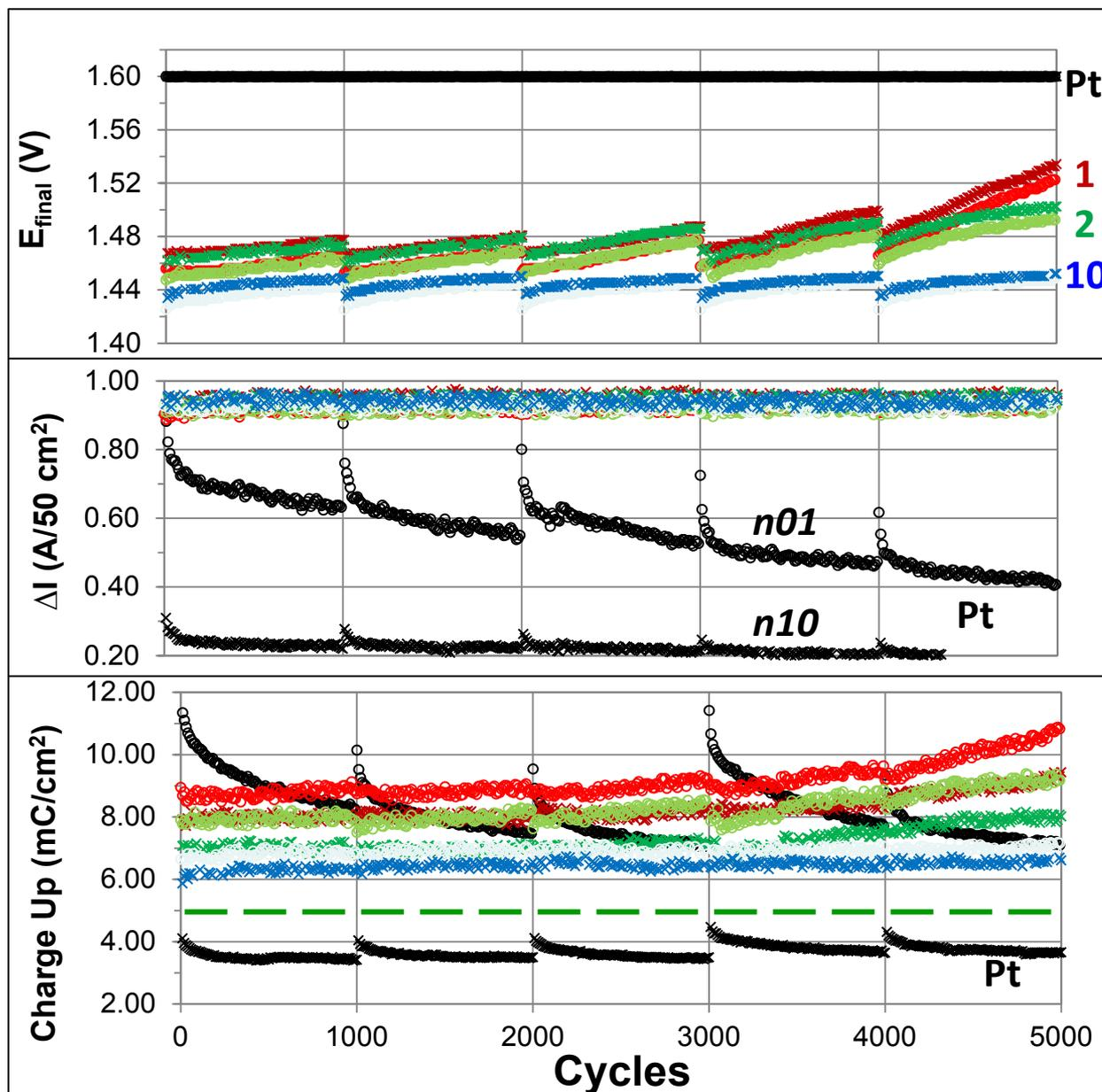
Note: Test done with current limit of  $1 \text{ A}/50 \text{ cm}^2$
