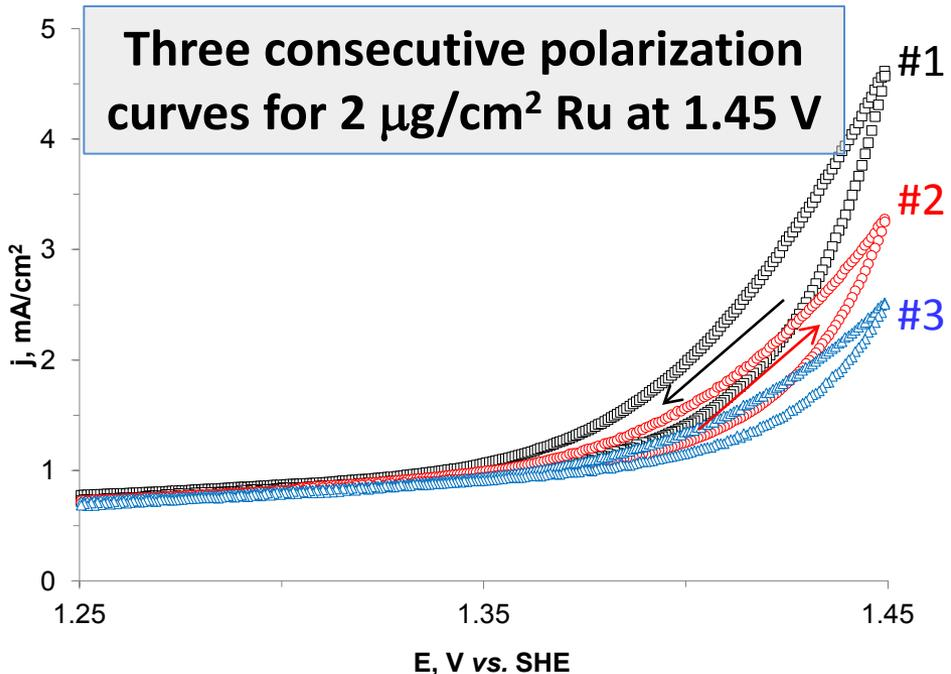
**Ru stability region:** overlapping of the negative going with the subsequent positive going scan: **1.40 – 1.42 V**
