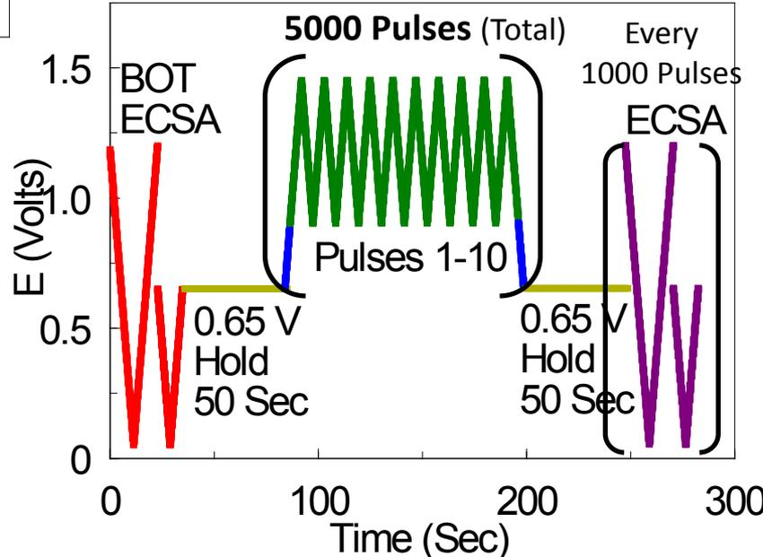
Go/No go SU/SD: 90  $\mu\text{g}/\text{cm}^2$  PGM total; New Protocol @ 100 mV/s, up to 1.6 V
