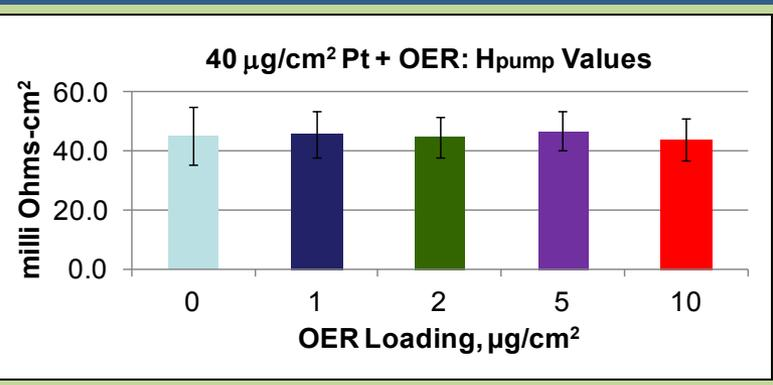
The OER added catalyst did not interfere with the normal HOR anode operation!
