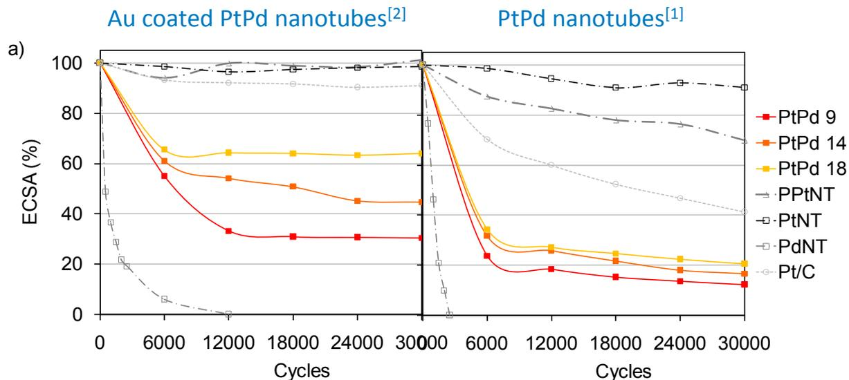
PtPd NTs and Au coated PtPd NTs investigated due to parallels with work of Adzic et al. and ability to be effectively investigated using SGD.
