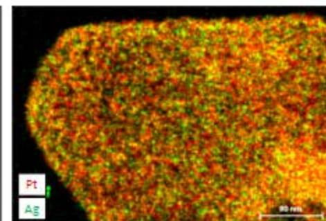
HR TEM consistently shows materials made up of agglomerates of small crystals/grains.
