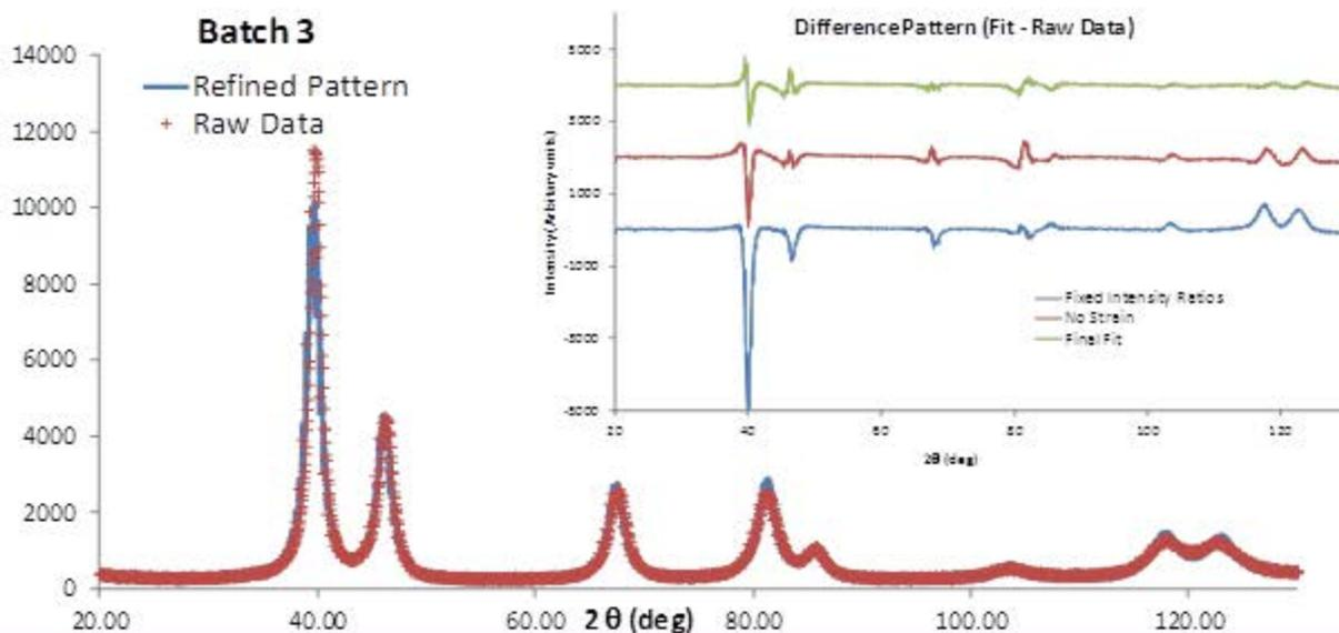
XRD fitting of catalysts show best fit with strain and preferred orientation, but are complicated and require further effort and technique refinement.
