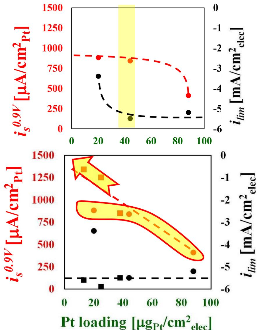
RDE limiting current can be a useful indicator of insufficient disc coverage, but particularly in the case of unsupported catalysts, does not guarantee a good dispersion.
