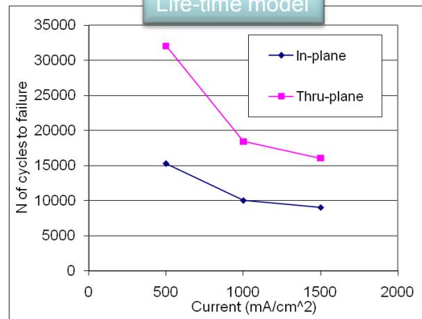
Developed modeling framework to relate fuel cell operation to membrane property changes and predict mechanical failure
