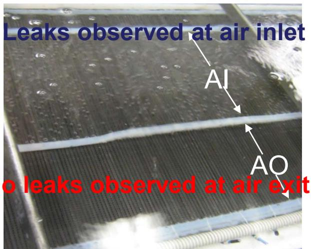
**Water submerge test showing air inlet**
