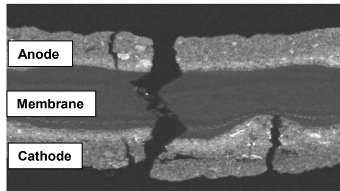
**SEM micrographs confirming membrane failure at the air inlet**
