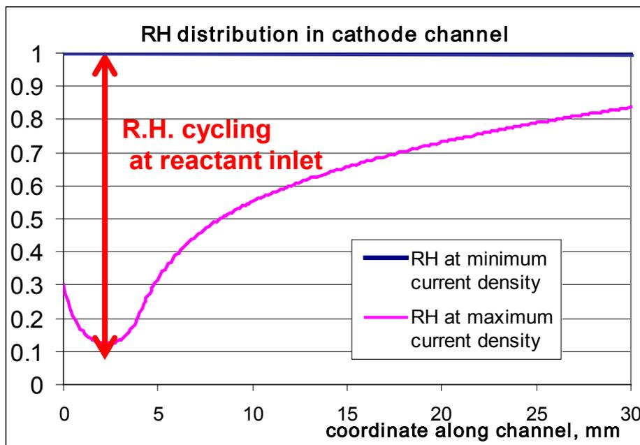
Model of Channel R.H. during load cycling
