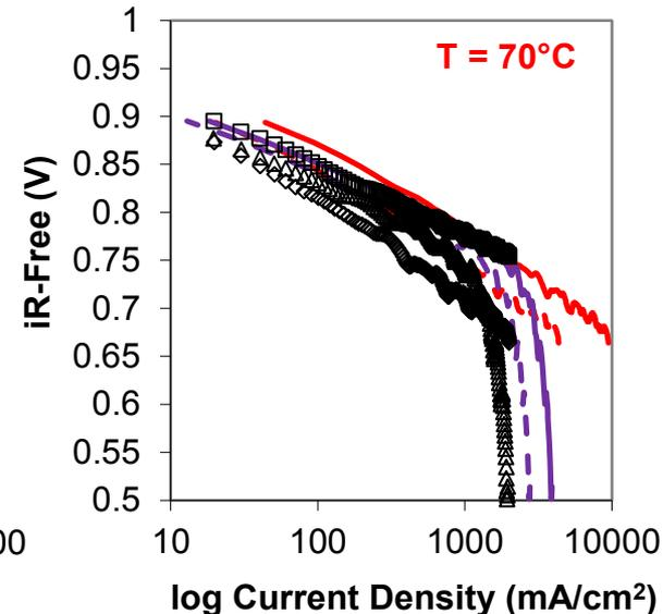
\* Oxygen gain shows external transport limitations at low temperatures
