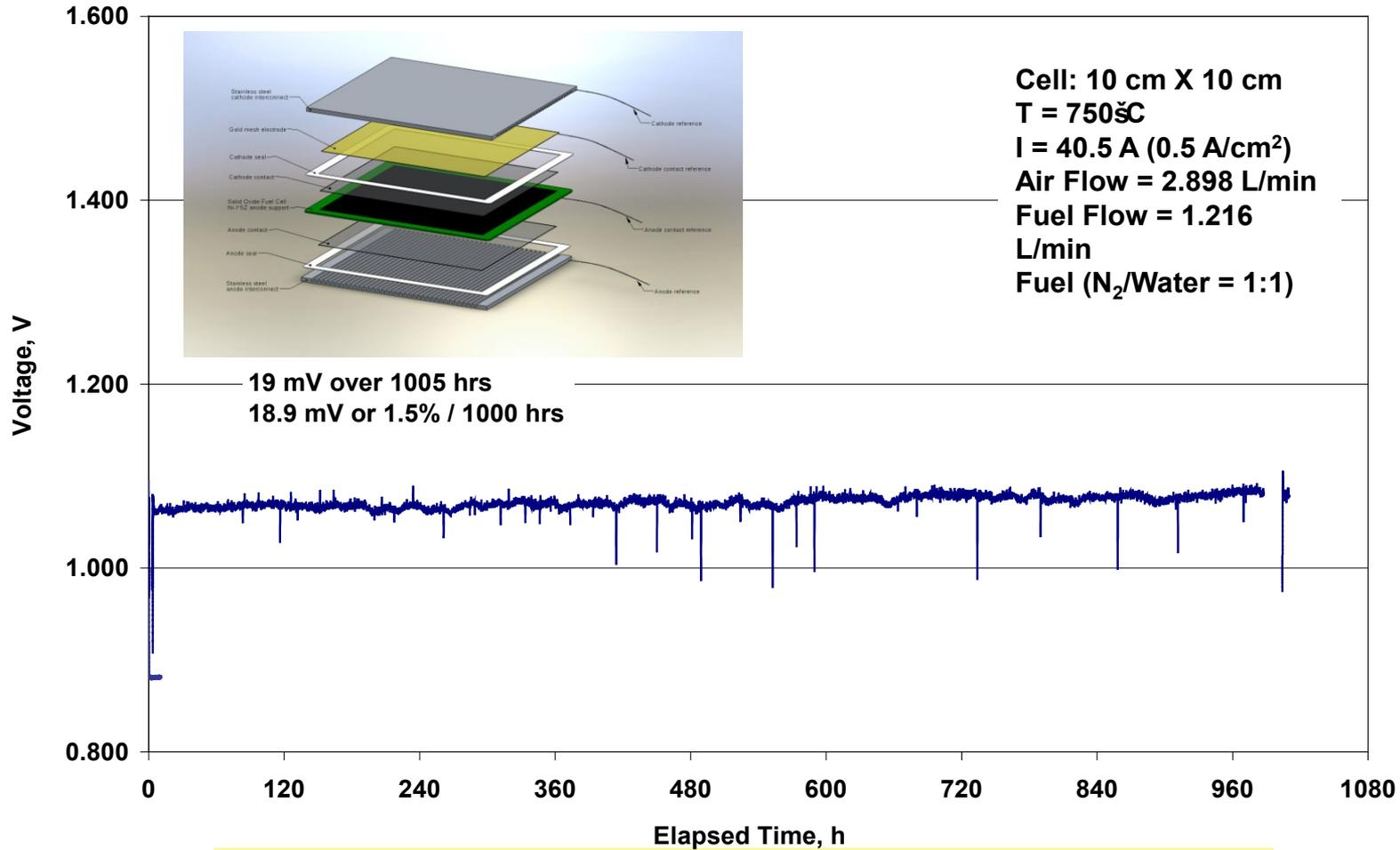
***Demonstrated electrolysis mode degradation of 19 mV, or ~1.5% per 1000 hours for the Go/No-Go Decision Test***
