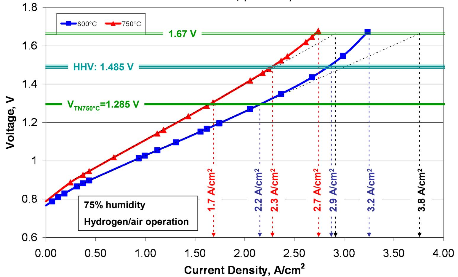
**High performance of RSOFC-7 can reduce hydrogen production cost and meet DOE water electrolysis efficiency (2017 target of 75%) at the same time**
