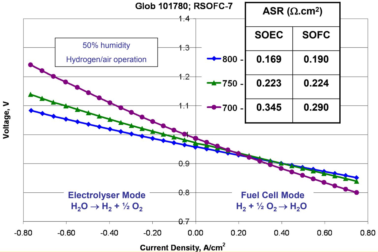
**High performance of RSOFC-7 can reduce hydrogen production cost in SOEC mode and improve efficiency in SOFC mode**
