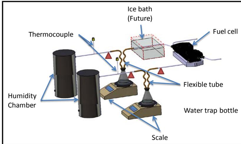
Water Balance experiment and numerical result of GM Down-the-Channel flow-field
