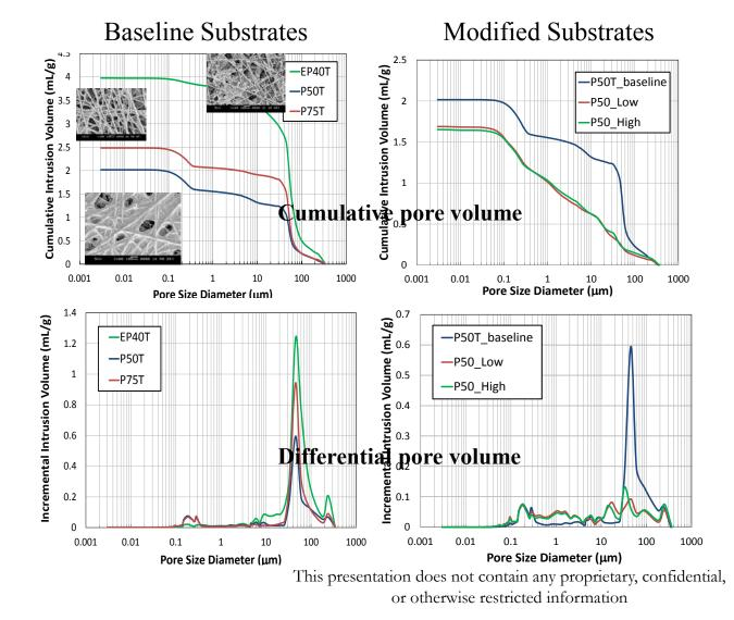
EP40T has largest pore volume, concentrated at 50 µm
