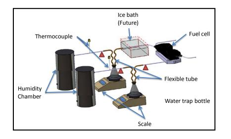
Water Balance experiment and numerical result of GM Down-the-Channel flow-field (<u>counter-current flow</u>: 50/50%RH, <u>101/101kPa</u>, 80°C, 1.5/2.0 stoich)
