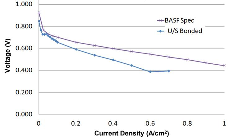
Average pol curves for thermally and ultrasonically bonded 140 cm<sup>2</sup> MEAs at 160°C, 1.2/2.0 H<sup>2</sup>/Air stoich, & old bipolar plates vs. BASF 50cm<sup>2</sup> MEA specification
