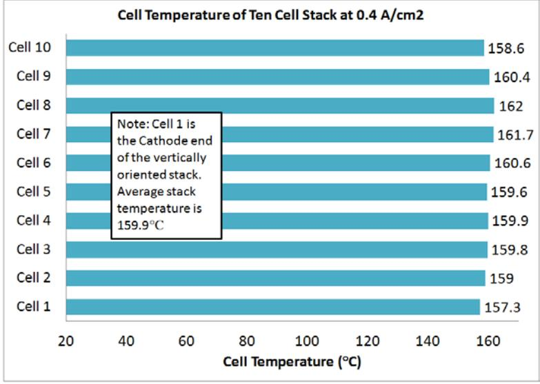
Temperature profile (bottom to top) of 10-cell stack with air,
