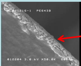
Varying pillar cross-section to simulate CCM roughness
