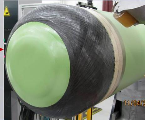
Repeated the first test but reduced to two tows instead of three on the first ply as well as reduced the steering on the first two plies.
