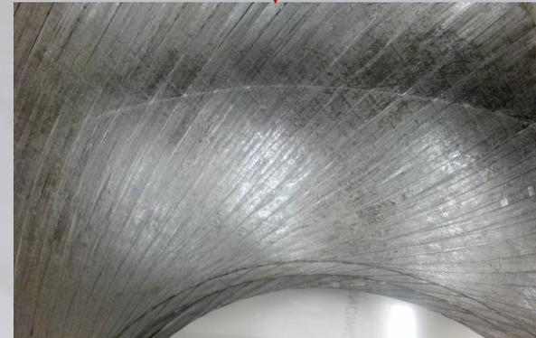
No visible wrinkling around the polar opening was observed. New standard process for domes.
