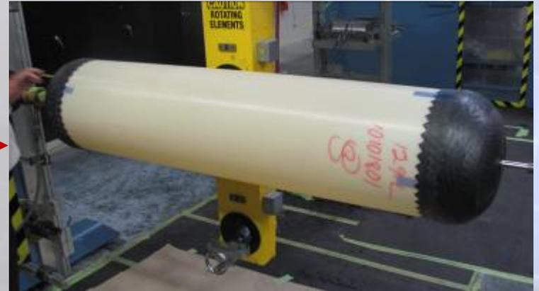
3. Both forward and aft dome caps are then transferred and installed to the hydrogen storage liner.
