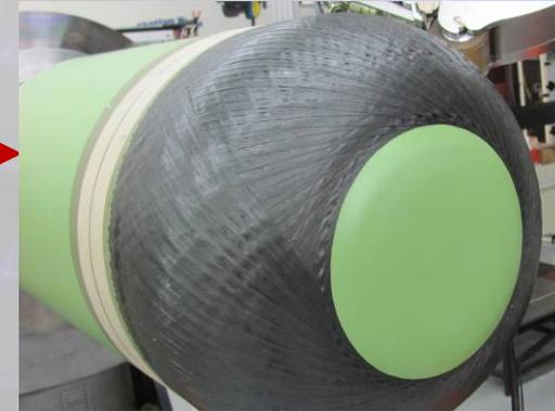
Sealed the foam tool surface to provide more secure surface for stretched FEP separator film.
