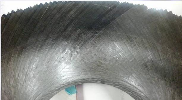
Wrinkling was still observed but was much less pronounced than was shown on previous layup with FEP. Attention turned to steering of first ply as being the cause.
