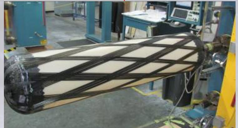
4. The final stage is to filament wound over the forward and aft dome caps.
