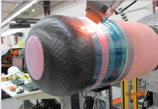
Process involves stretching FEP (fluorinated ethylene propylene) film over tool surface. Poor control of FEP over machined foam could result in material movement causing issues.
