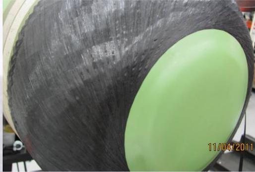
Next, the FEP liner was removed and dome laid directly up on the sealed surface with original 3 tow layup having steering on first few plies.
