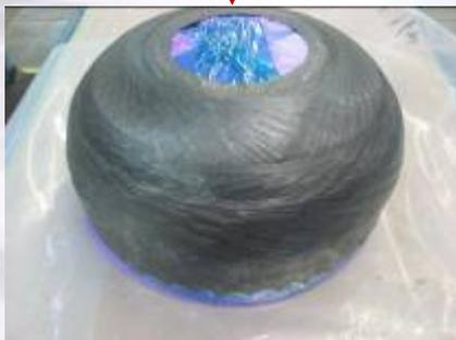
2. AFP dome caps (forward and aft) are then removed from foam tooling and brought to wind cell.
