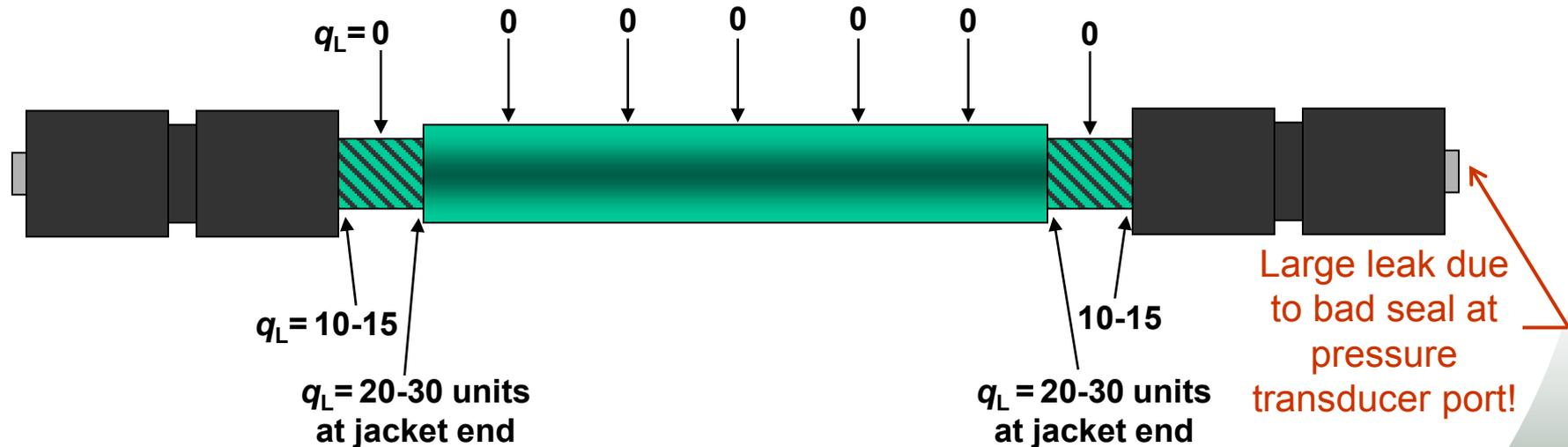
H<sub>2</sub> detected at jacket ends and end joint connectors
