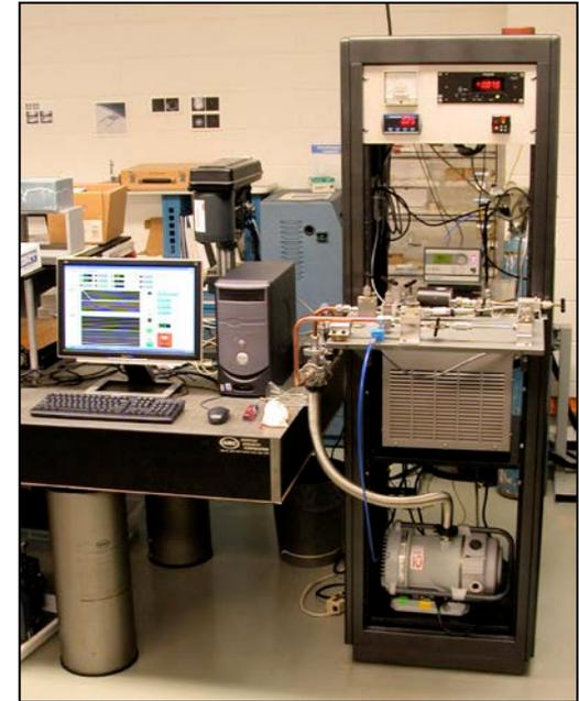
Measurements of  $D$  and  $P$  at  $T = -40$  to  $85^\circ\text{C}$ ,  $p \leq 480$  bar (7000 psi)
