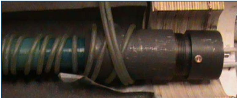
Pipeline joint connector with end cap
