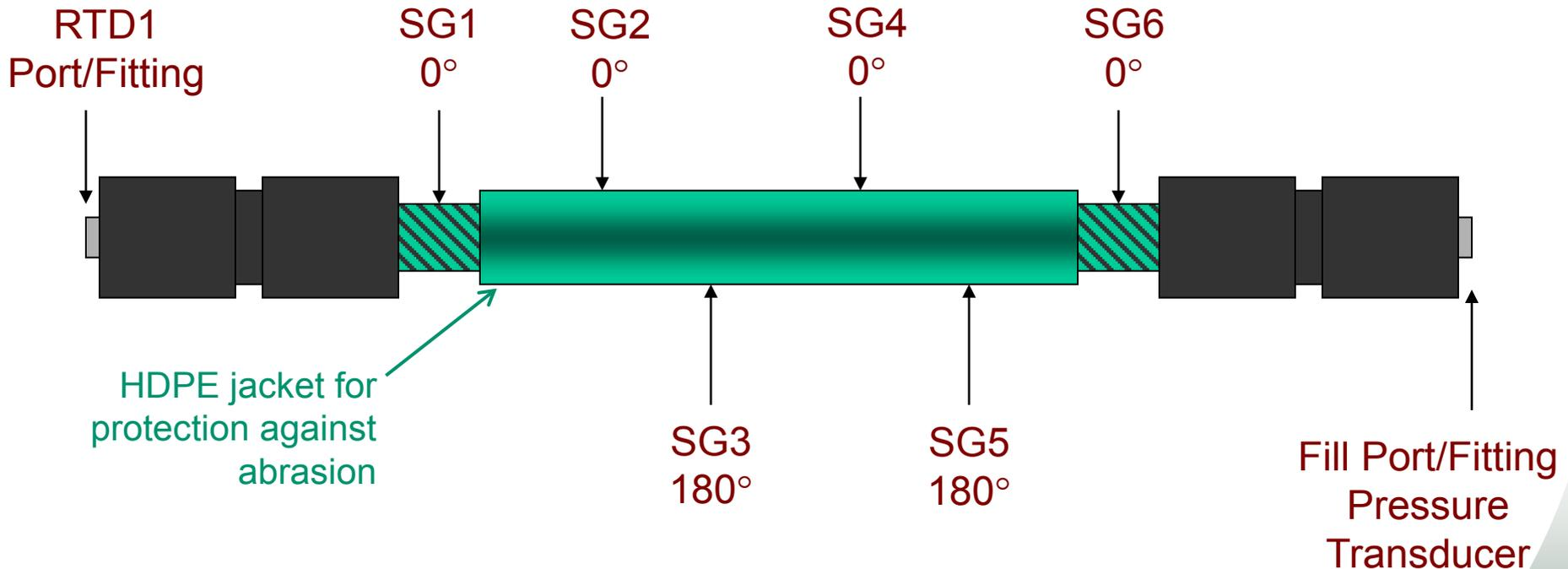
Slight residual curvature in pipeline (due to its storage on spool prior to testing) prevented useful longitudinal strain measurements
