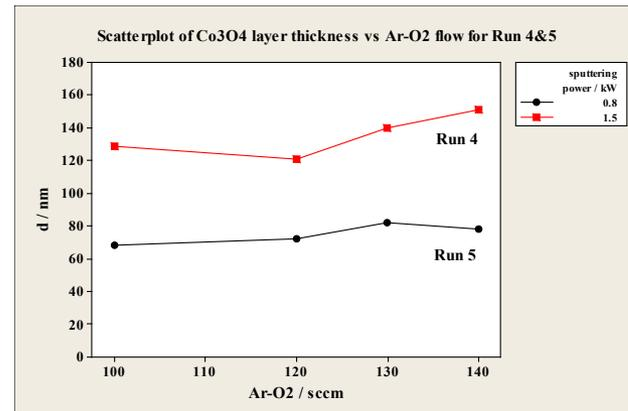
Fig. 2:  $\text{Co}_3\text{O}_4$  thickness vs. Ar- $\text{O}_2$  flow:
