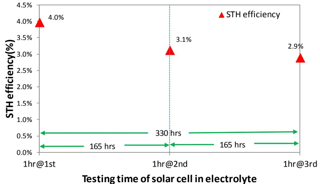
*Solar to hydrogen conversion efficiency for PEC electrode with cobalt oxide TCCR coating at the oxygen generation side and platinum coating at the hydrogen generation side. Corrosion of clear coat at edge of the cell likely is the main reason of the STH decrease. The PEC electrode is still under testing...*
