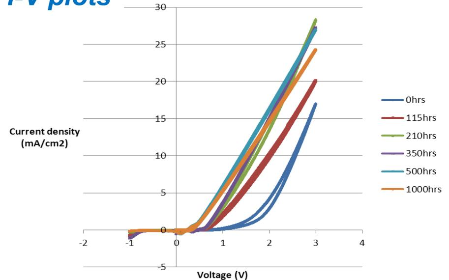
*IV-plots show little to no change after biasing in electrolyte (115hrs-1000hrs); the drift between initial and 115hrs measurement is caused by oxidizing residual metallic Co in the film;*
