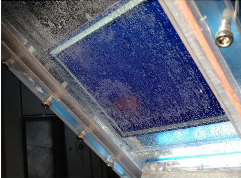
A PEC module with a 1.5"x1.5" electrode produced 4 ml of O<sub>2</sub> and 8 ml of H<sub>2</sub> in 90 min.  $P = 100 \text{ mW/cm}^2$ .
