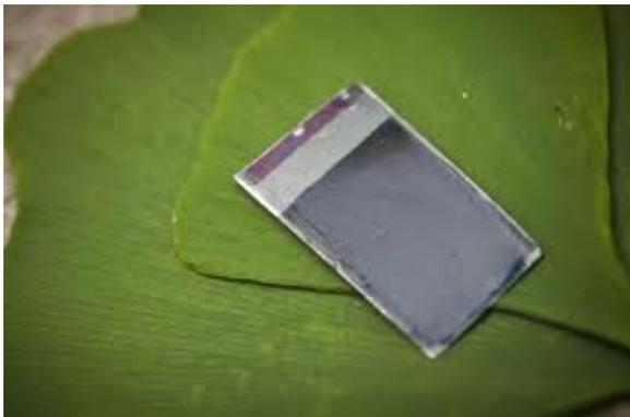
*"Artificial Leaf" by Dr. Nocera's MIT lab made use of MWOE/Xunlight's triple junction a-Si solar cells*
