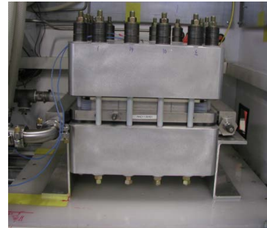
Existing large format stack scaling to >50-cell design point
