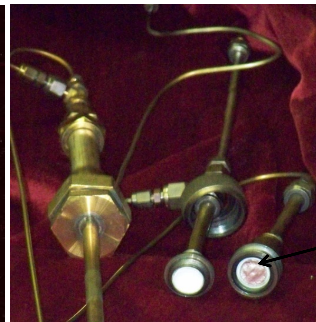
Pd Alloy Discs after 34 Cooling Cycles: Pd-Cu was intact, Pd-Ag showed wrinkle near the edge, Pd and Pd-Au failed.
